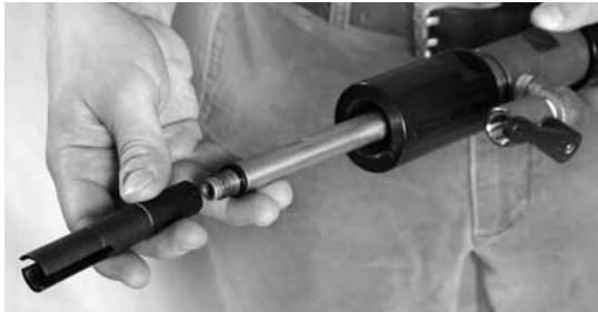
Attach coupling nut to shell cutter.
