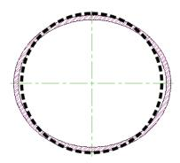
The ends of HDPE can experience an "egging or necking down" and be out of round beyond mechanical fitting tolerances.
