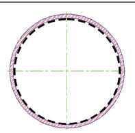
Installation of stiffeners brings pipe "into round" and provides a rigid support for mechanical fitting installation.
